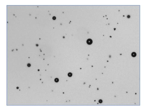
Toner grains are small, with a low quantity of larger beads in occurrence, and are almost spherical. As it is legitimately possible to presuppose universal sphericity, it is enough to implement Equivalent Circular Area as the predominant size measure, alongside Circularity and Smoothness, which yield further characterization.
