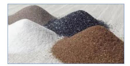
Predictably, the more aggressive the grit, the more efficiently the material is removed. However, the powder's grit is not only determined by the size of the particles, but also its shape properties. A low grit, corresponding to a more robust removal, has larger particles. Nevertheless, if these larger particles were all smooth and round, the removal effectiveness would be weak. Consequently, both size and smoothness are key factors in the performance of abrasive powders.
