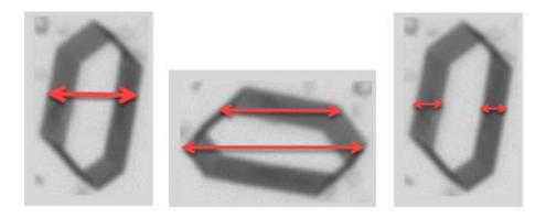
In some instances, the refractive index difference of the carrier fluid versus the translucence of crystal particles can have adverse effects on rendered size values where just the particle's crystal edges are measured.
