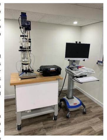
analysis of the raw material is carried out "on-line", next to the reactor or process. As it is portable in nature, the Pi Mobile can be easily disconnected from one process and reconnected to another without any disruption. To ensure minimal dead-volume from the process, the analysis module is connected via a tether allowing it to be close to the process while the control unit can be out of the way offering the user unobstructed access to the process.
