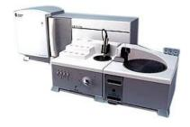
The LS 13 320 Laser Diffraction Particle Size Analyzer uses laser diffraction and the patented polarization intensity differential scattering (PIDS) technology to rapidly determine the particle size distribution of materials with an overall sizing range of 0.04  $\mu m$  to 2000  $\mu m$  in a single scan with no extrapolation. This is accomplished with high resolution and excellent reproducibility.
