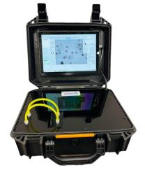
The **Portable Particle Insight System** is a full-featured laboratory particle size and shape analyzer utilizing Dynamic Image Analysis technology. Housed in a ruggedized case with battery operation allows for laboratory as well as remote field use.
