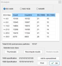
The **Wear Classification function** allows the user to view statistics, statistical listing, and particle thumbnails for each desired type of particle >1 $\mu$ m. Wear classifications can be adjusted to meet users needs. Additional custom classification types can also be created.
