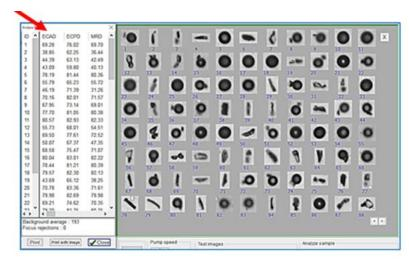
**Thumbnails** shown in greyscale view to enhance users understanding of all particles starting at 1µm.
