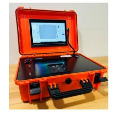
The **Portable Particle Insight System** is a full-featured laboratory particle size and shape analyzer utilizing Dynamic Image Analysis technology. Housed in a ruggedized case with battery operation allows for laboratory as well as remote field use.
