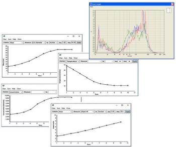
**Result overlays** allows comparing results by shape, not just size. Smoothness, or circularity are common non-size related measures that can impact flowability of process particles.
