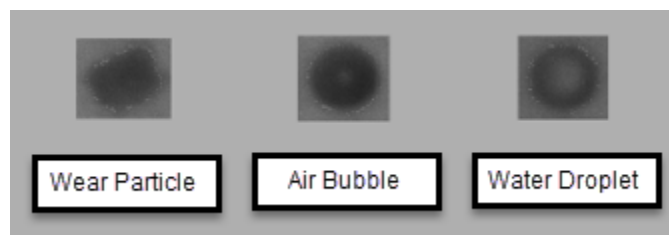
Figure 7 - Ensuring identification and differentiation between particles, air bubbles, and water droplets down to 1 micron in size.
