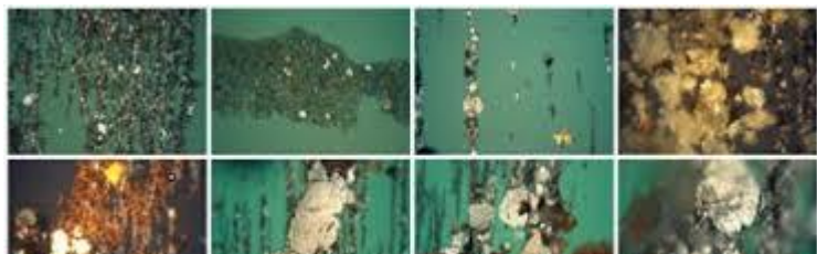
Figure 3 Examples of wear types from the Noria Wear Atlas. This was used to create classifications on the Raptor system.
