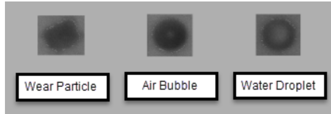
Figure 4 Dynamic Imaging uses the shape of each particle to differentiate them.
