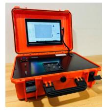
The Particle Insight Raptor Portable for Fluid Analysis is designed to perform high resolution precision measurements of detected particles from 1um to 100um in a portable and benchtop configuration. By using Dynamic Image Analysis and a flexible sampling design users can get a full picture of machine war and contamination. Unique Features include:
