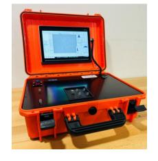
The Particle Insight Raptor Portable for Fluid Analysis is designed to perform high resolution precision measurements of detected particles from 1um to 100um in a portable and benchtop configuration. By using Dynamic Image Analysis and a flexible sampling design users can get a full picture of machine war and contamination. Unique Features include:
