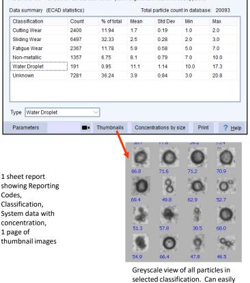
detect unimportant particles such as air bubbles.
